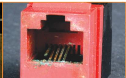
Humidity corrodes contact pins inside typical outlets. Repeated exposure can eventually destroy the contact pins, rendering the outlet unusable. The Ruggedized MAX outlet's special housing prevents this corrosion.
